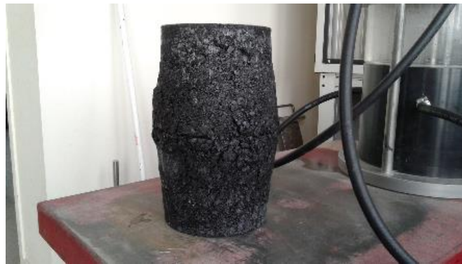
FIGURE 4 Repeated Load Triaxial Test result on AC20 with 40/50 binder Asphalt Cylinder at 40 degrees celcius after 200 cycles for a 30 second haversine load pulse (vertical load of 550kPa).
