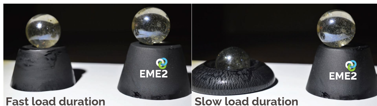
Figure 6: Viscoelastic response with varied load duration
