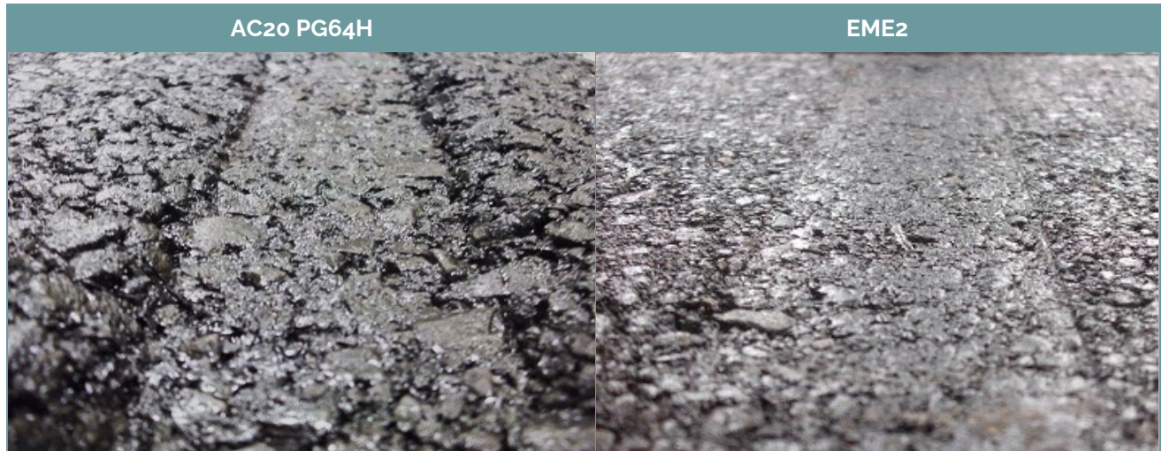
Figure 2: Wheel Track Roller Comparison
