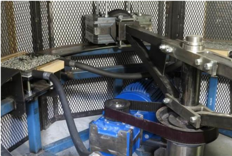
Figure 1: CAST machine used to apply repeated loading to chip seal test samples (Reproduced from Circular Accelerated Surfacing Tester (CAST) for Evaluating Chip Sealing Binders ).
