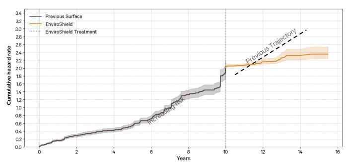
Estimating the service life of new products is challenging, as most treated surfaces have not yet required resurfacing indicating product failure. Of the 195 roads monitored, none have undergone resurfacing to date. However, using faults as a failure criteria we can create a survival probability of time to first fault – this is quite conservative as the fault may be an isolated occurrence.
