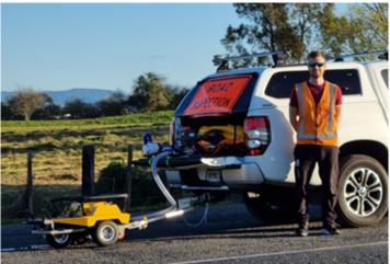
Images: (left) GripTester MK2 completing airfield friction testing. (right) GripTester MK2 on-site road inspection for skid resistance.
